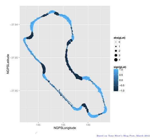
We should be able to see from the plot the forces on the driver on the left and right hand corners, and see how tight the corner is based on the size of the dots.
